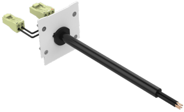
Dry Location Power Connector (18/5 Gauge Wire) (ALS600T-PC-DRY-X) X = Specify Length
