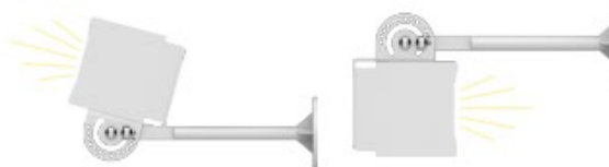
Tilt either direction in 15° increments. Minimum Tilt: -105° outward, away from mounting surface Maximum Tilt: 90° inward, toward mounting surface
