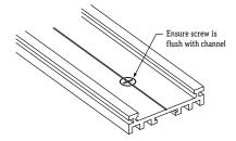
4. Remove adhesive backing from lightstrip, then install into channel.
