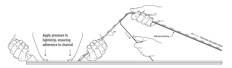
One person on one end applies pressure to LLED8550, securing it to channel
