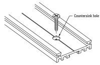
3. Screw channel into desired surface using countersink holes. **NOTE:** Surface must be flat.
