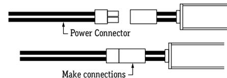
2. Perform continuity test before connecting fixture to power source.
