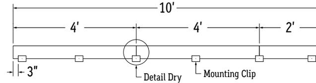
5. Lay mounting clips and pre-drill using proper drill bit for surface and screw size.
